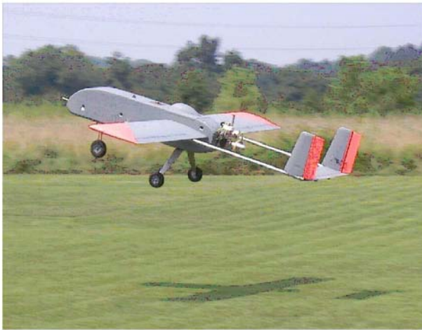
Figure 2. An unmanned aerial vehicle (UAV) is taking-off from a grass runway. The UAV, developed by Intellitech Microsystems, can carry a variety of remote sensing instruments and can be programmed to acquire images over agricultural fields to assist crop scouting.
